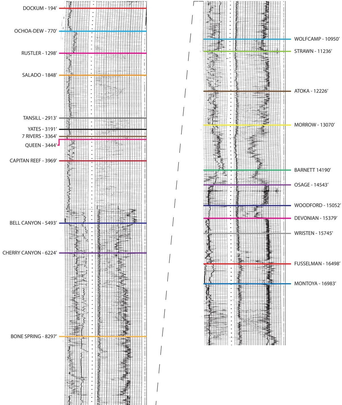
Figure #&. Type log of nearby well (API #30-028-25046) illustrating identified formation tops. Estimated formation tops for the proposed section 20 Ameredev AGI location are included in Table 6.
