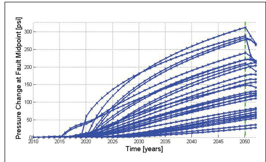
**Panel C.** Model-predicted pressure change through time at the midpoint of each fault segment included in the simulation
