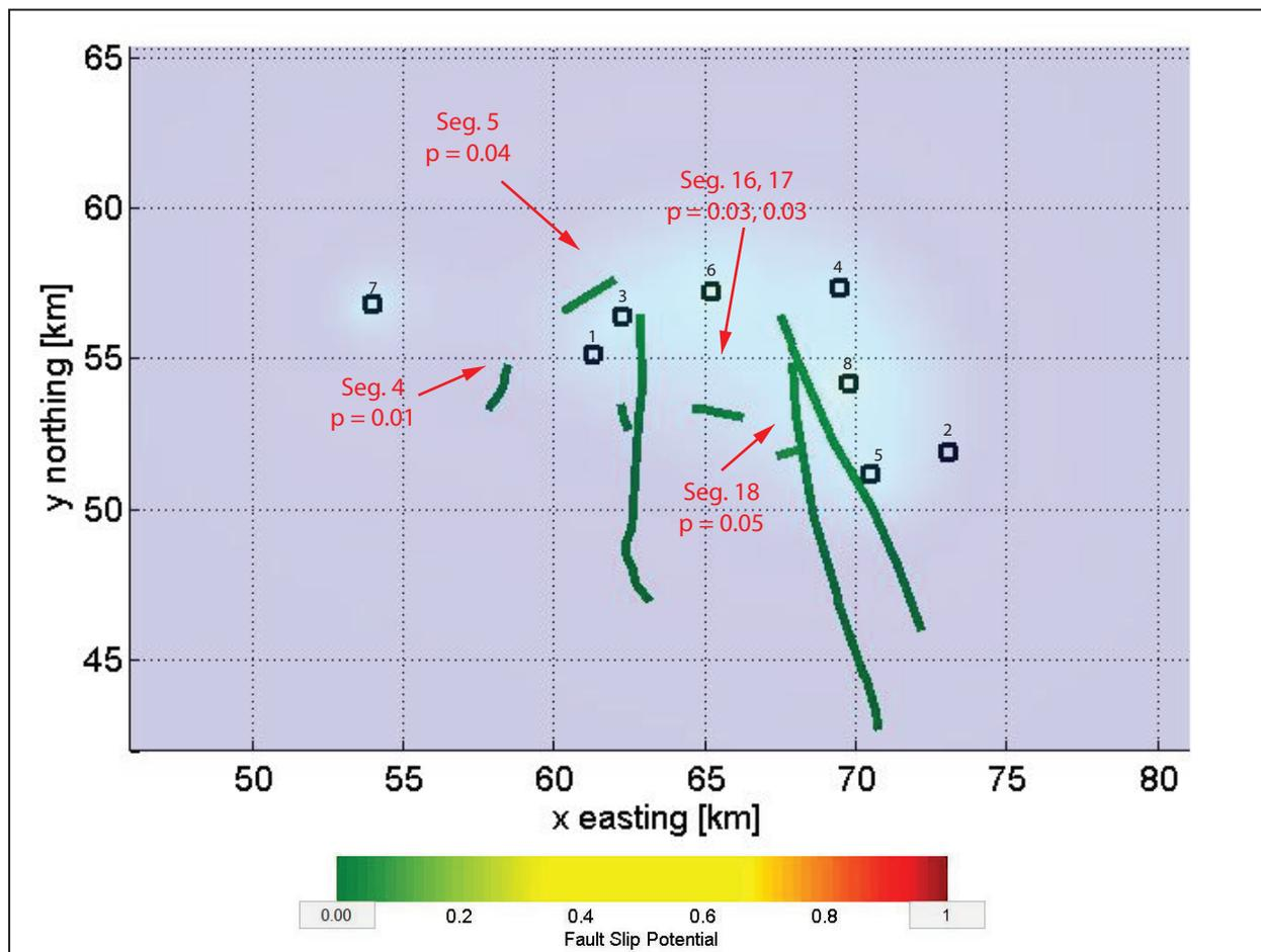
**Panel B.** Map view illustrating the model-estimated slip potential of faults at the end of the 40-year injection scenario. Any feature estimated to have a non-zero slip potential determination has been labeled on the above map.
