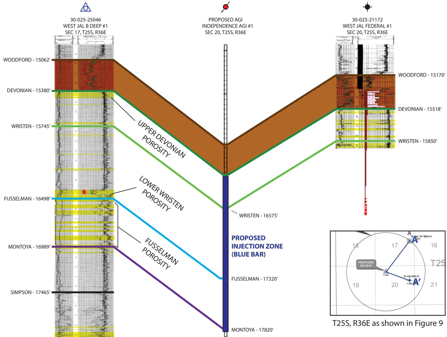
Figure 1 (. Structural cross section A - A' showing porosity profile from nearby offset wells penetrating the proposed injection interval and regional extent of overlying Woodford Shale caprock. Proposed injection zone from 16,230 feet to 17,900 feet (blue bar).
