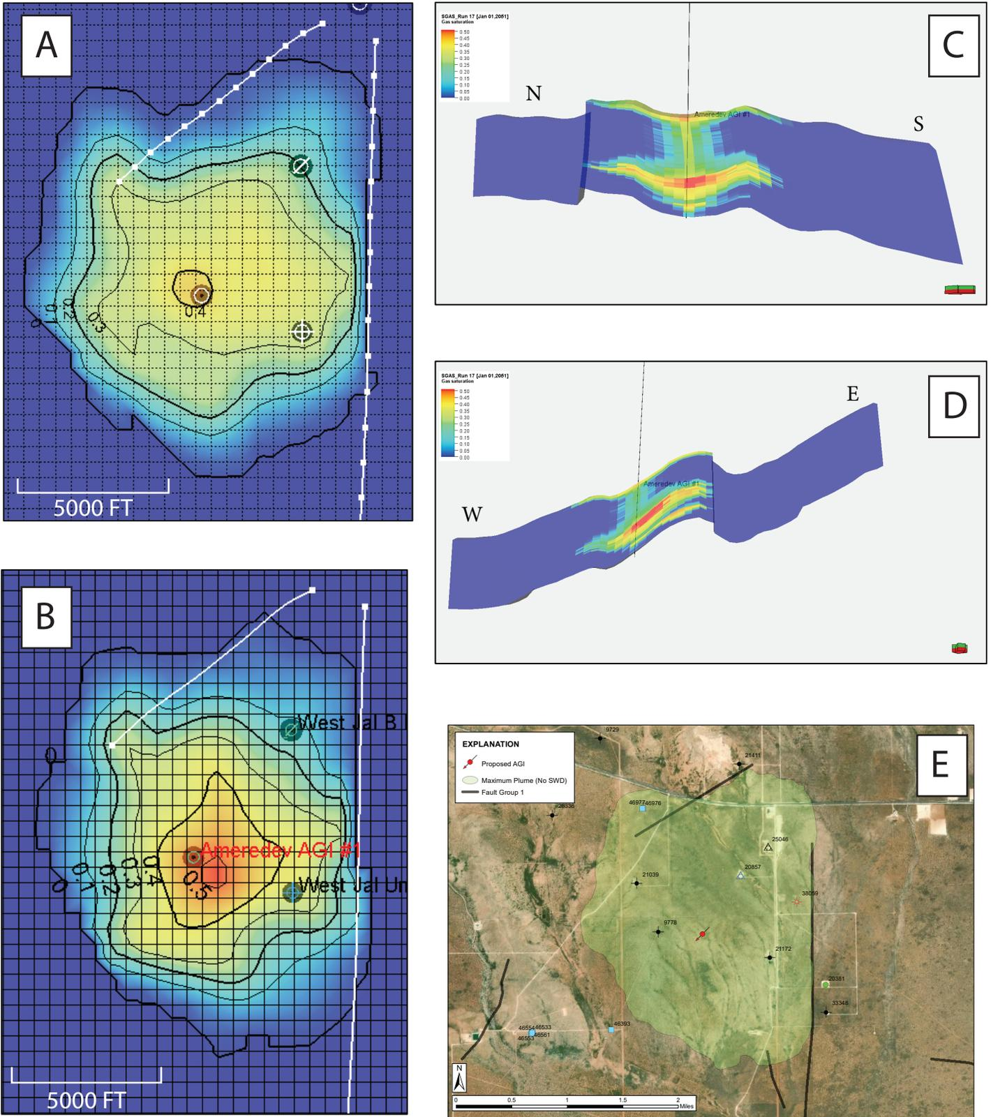
Figure 8. Summary of ECLIPSE injection simulation results when West Jal B Deep #1 is not actively injecting. Panels A and B include gas saturation maps for identified zones 1 and 5; panels C and D illustrate cross-sectional view of the resultant injection plume; panel E illustrates combined zone 1 and zone 5 plume footprint.
