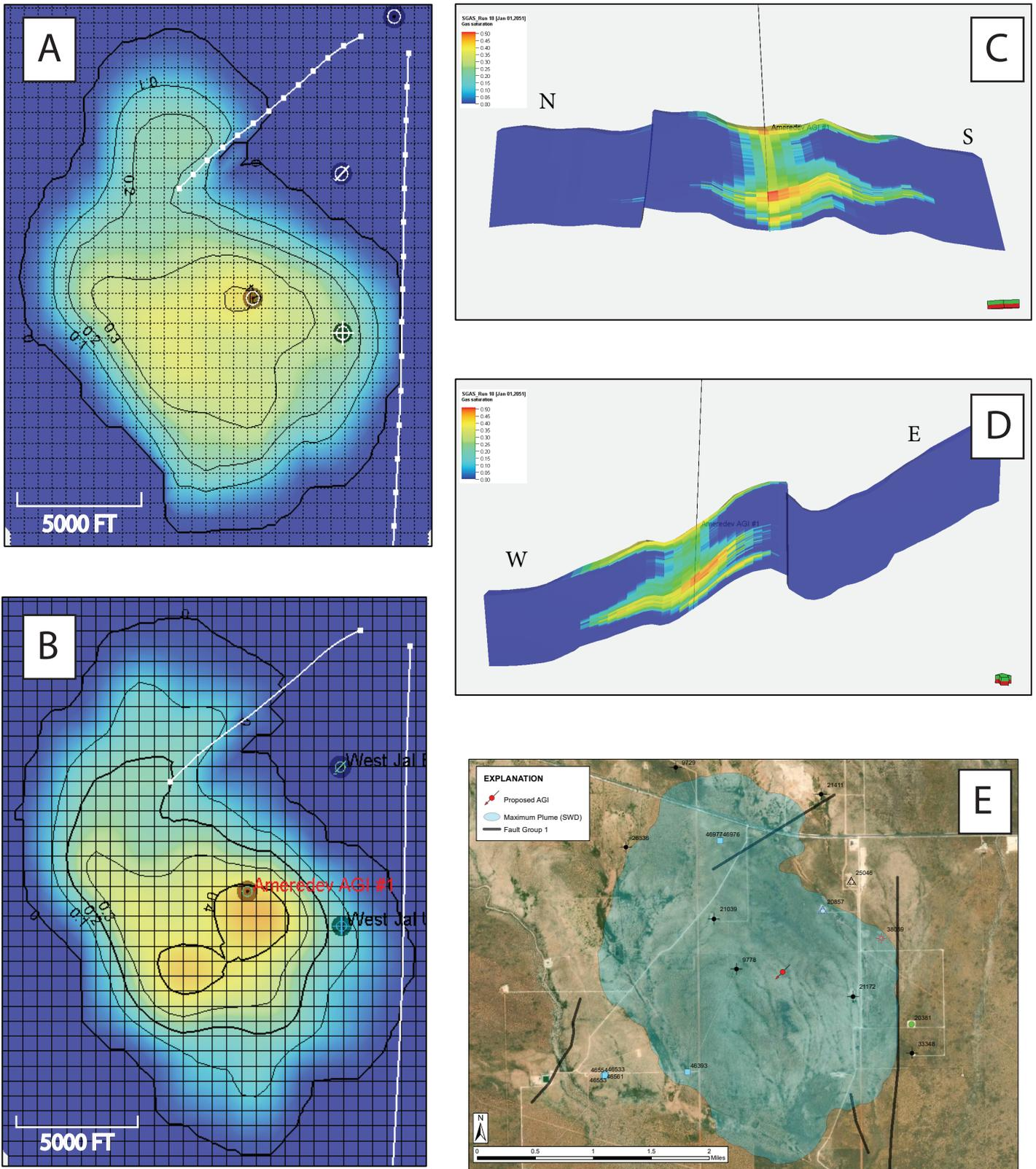
Figure 9. Summary of ECLIPSE injection simulation results when West Jal B Deep #1 is actively injecting. Panels A and B include gas saturation maps for identified zones 1 and 5; panels C and D illustrate cross-sectional view of the resultant injection plume; panel E illustrates combined zone 1 and zone 5 plume footprint.
