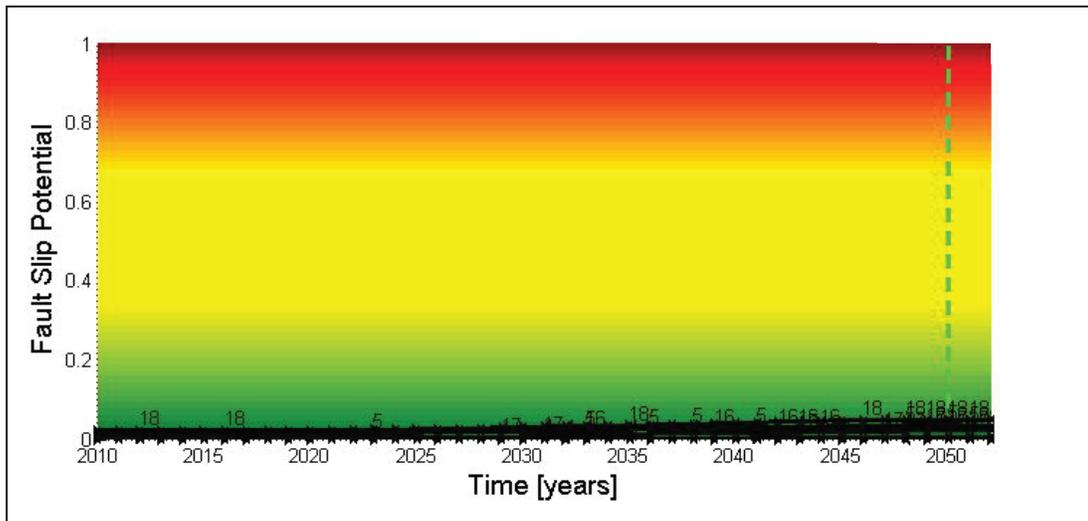
**Panel A.** Fault-slip probability throughout the entire simulated injection period. FSP model results suggest no significant risk of injection-induced slip along any feature included in the simulation.
