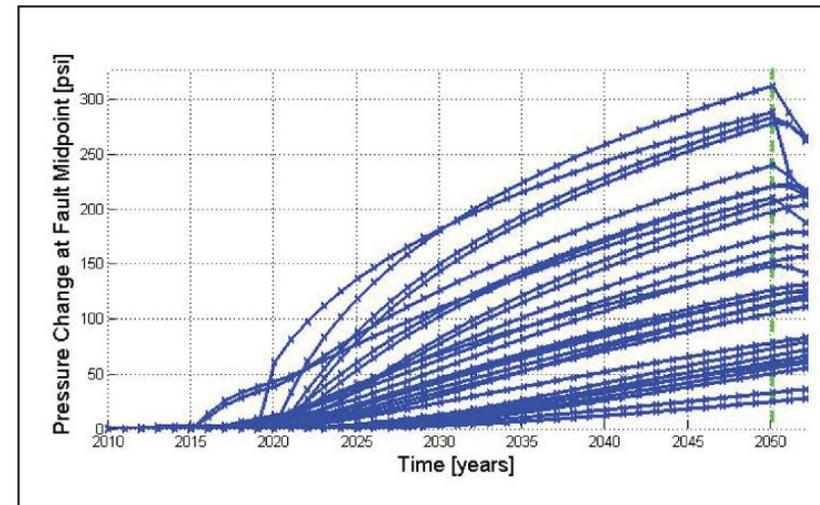
Pressure change experienced at each fault segment throughout the simulated injection scenario
