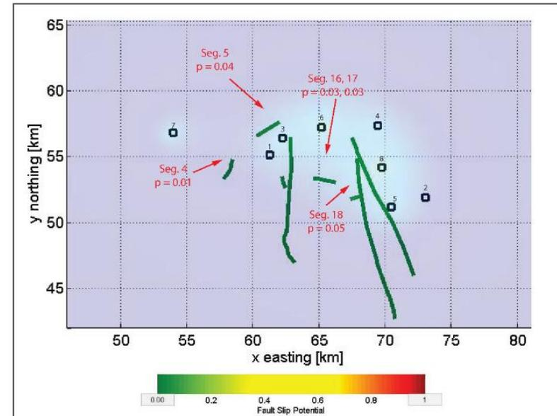
FSP fault map annotated with non-zero model predictions of slip potential
