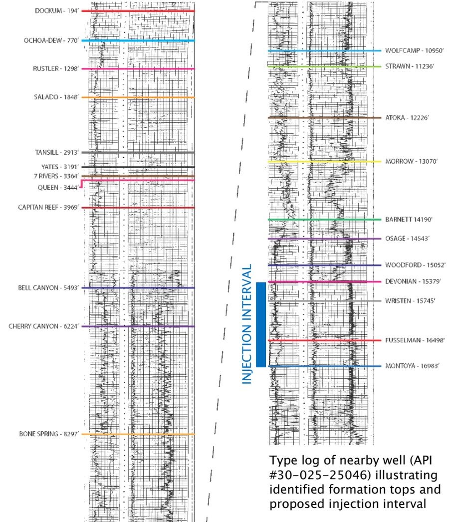
Type log of nearby well (API #30-025-25046) illustrating identified formation tops and proposed injection interval
