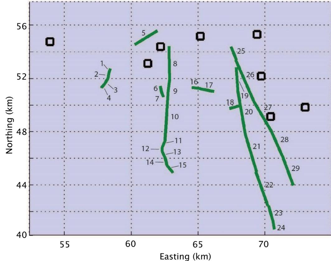
Subdivision of eight identified faults into 29 fault segments for simulation
