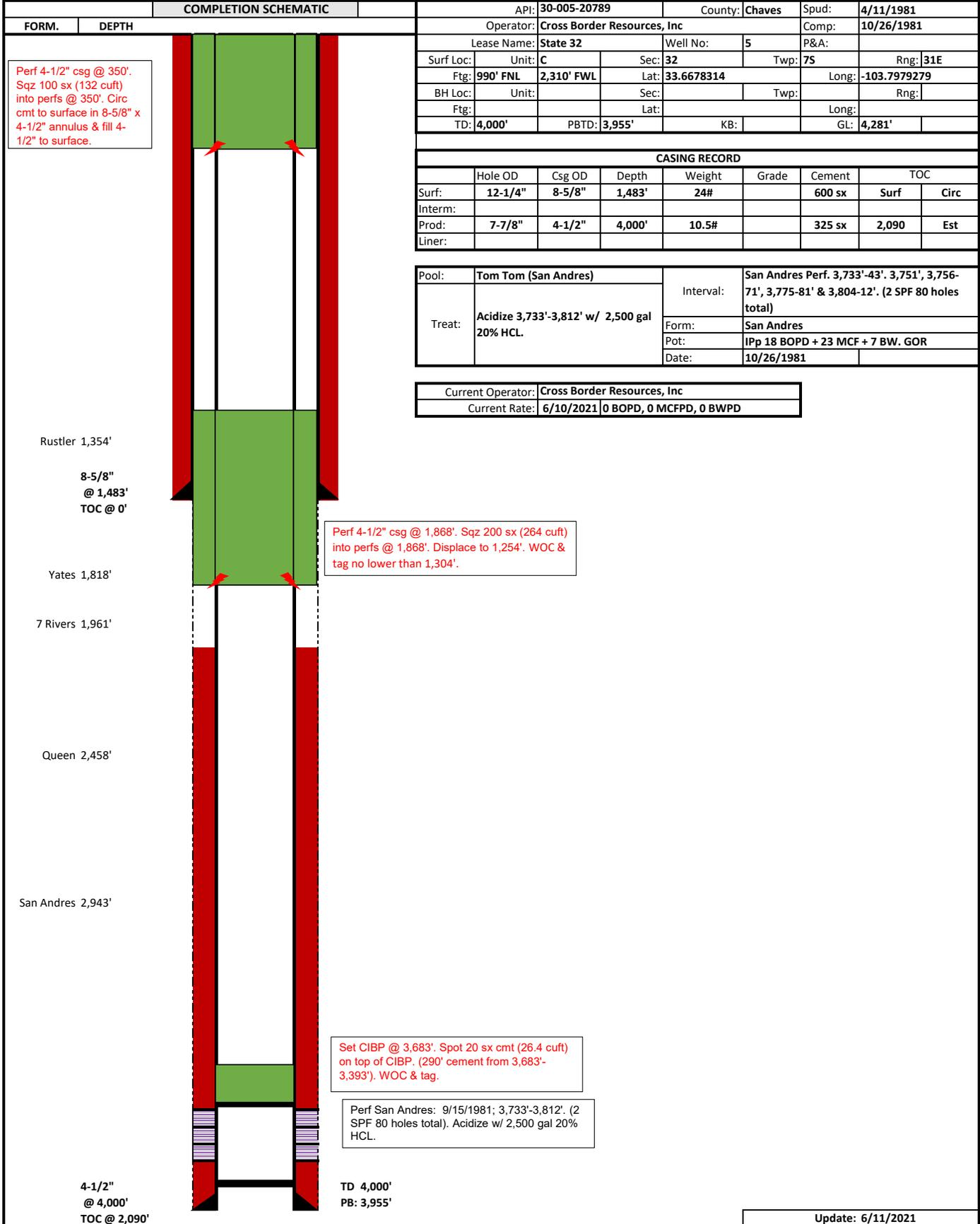
Perf 4-1/2" csg @ 350'. Sqz 100 sx (132 cuft) into perms @ 350'. Circ cmt to surface in 8-5/8" x 4-1/2" annulus & fill 4-1/2" to surface.
