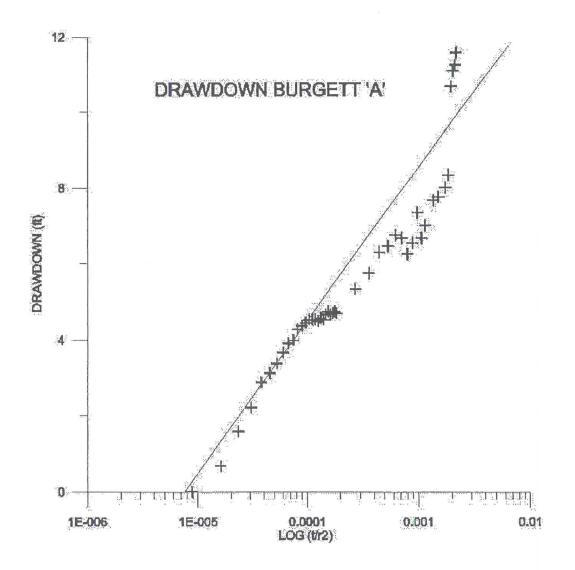
Twenty-Four hour drawdown for the Burgett 'A' well 825 feet from the pumping Americulture 1 State well. Pump rate was steady at 1, 000 gpm in the Americulture production well. The graphed line is the drawdown slope that was used to calculate reservoir transmissivity and storativity with the Cooper and Jacob method. The axis labeled  $log(t/r^2)$  is the log of the ratio of time (in minutes) and radial distance (in feet) from the pumping well.
