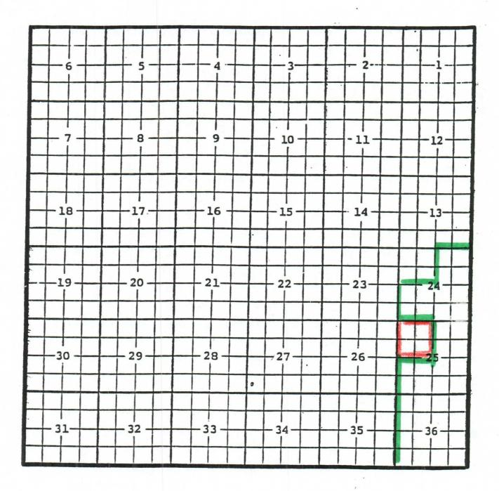
Purpose: One completed oil well capable of producing. Devon Energy Production Company, Apache '25' Federal # 4 Location: Unit A, Sec. 25, Township 22South, Range 30 East, NMPM Completed 03/23/05 in the Delaware formation Top of perforations: 8066'.
