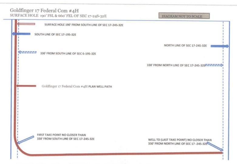
\*No perforations will be performed closer than 330' from the section lines.
