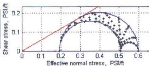
Vertical fractures striking ~N50°E and N°110E start to slip (green circles).
