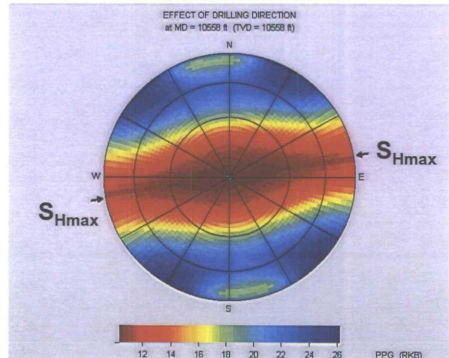
The plots show fracture initiation and link-up pressures as a function of deviation and azimuth. The plots indicate that both deviation and azimuth have an effect on fracture pressure. A horizontal well drilled in the  $S_{Hmin}$  direction (~N-S) requires much higher pressure to link up or initiate fracs than a horizontal well drilled in the  $S_{Hmax}$  direction (~E-W).
