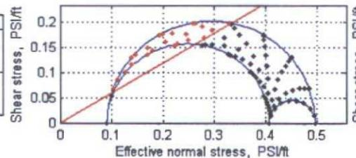
Fractures striking N40°E – N120°E with 50-90° dip angle (poles within the green circles (white dots)) are optimally oriented to slip and become permeable.
