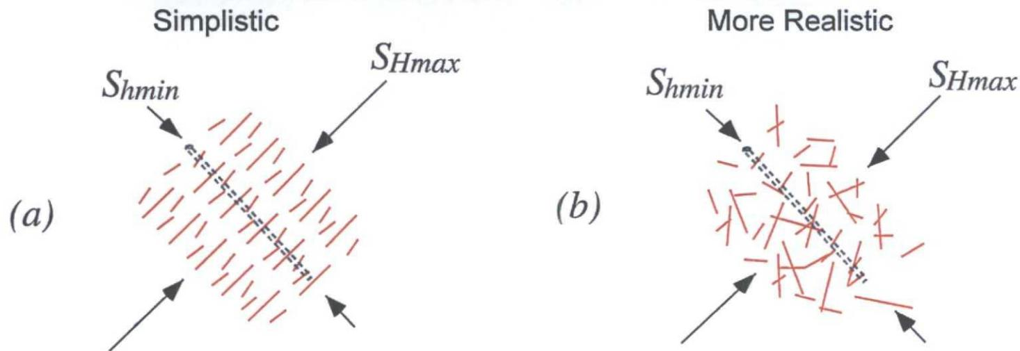
Permeable Fractures and Faults are Critically Stressed
