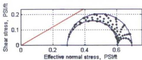
No fractures are critically stress under current stress state.
