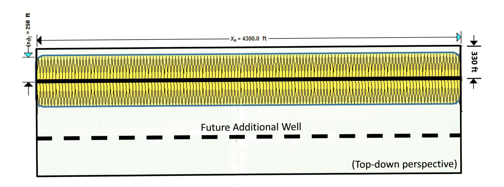
330' from the lease edge allows for more efficient recovery of hydrocarbons.
