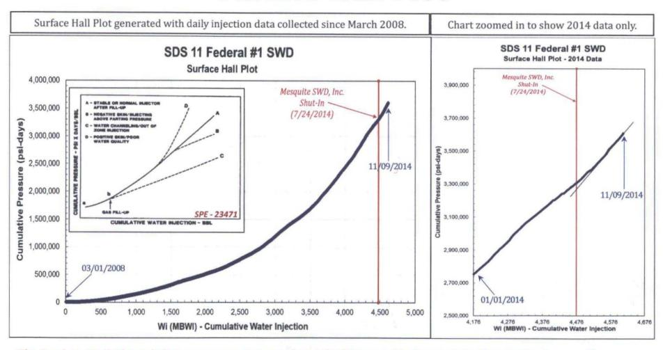
The Surface Hall Plot exhibits a <u>concave upward</u> trend. This trend indicates injection under "normal" conditions, or reduced injectivity over time.
