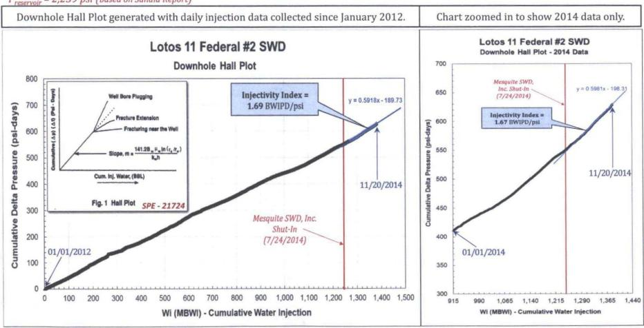
The Downhole Hall Plot primarily exhibits a <u>linear</u> slope, which indicates injection under normal conditions. Injectivity Index is calculated as the inverse of the slope (steeper slope yields smaller I.I.).
