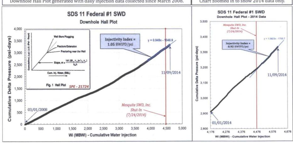
The Downhole Hall Plot primarily exhibits a linear slope, which indicates injection under normal conditions. Injectivity Index is calculated as the inverse of the slope (steeper slope yields smaller I.I.).
