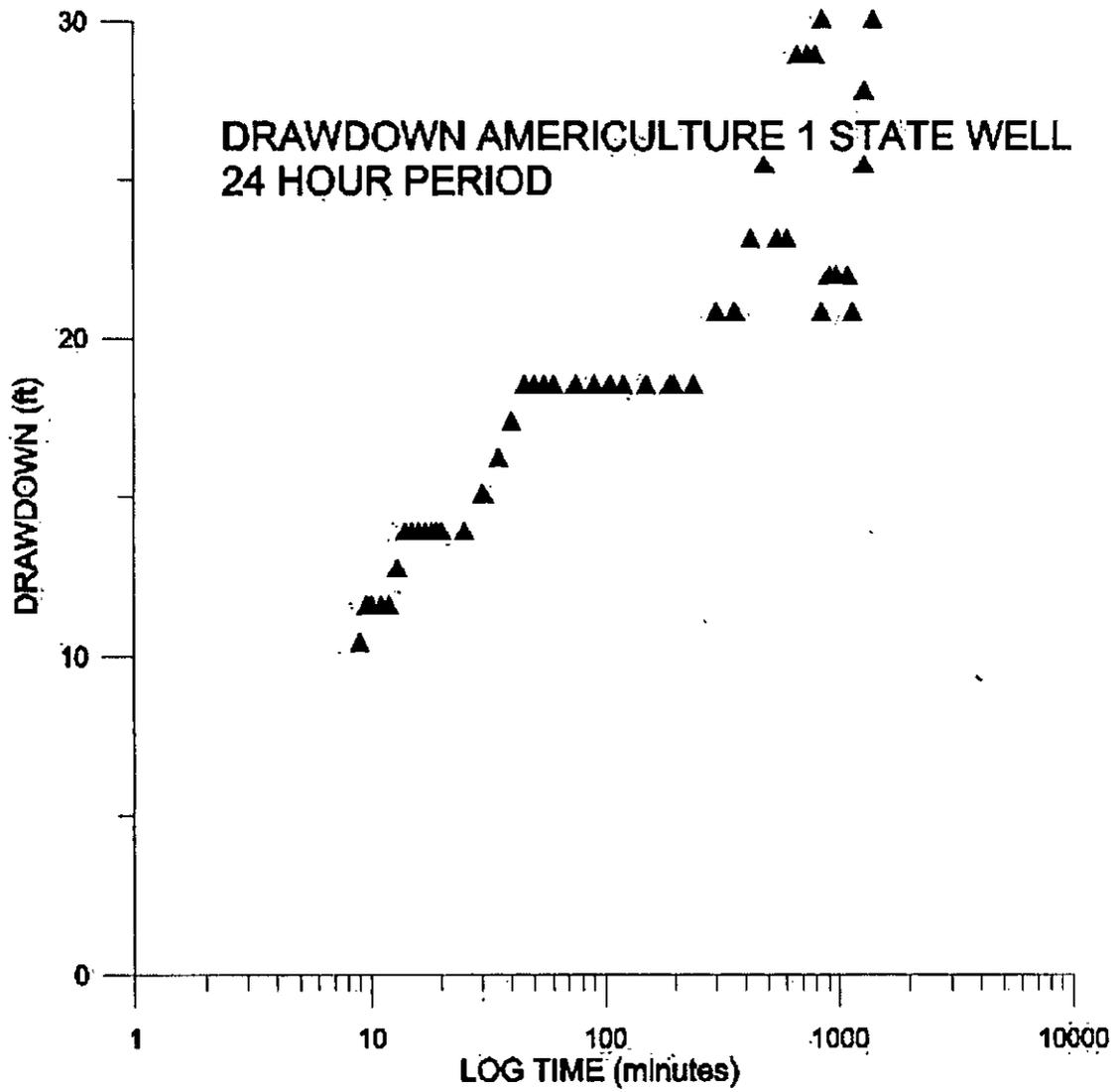
Figure 8. AmeriCulture 1 State pumping well twenty-four hour drawdown. Continuous pumping rate is 1,000 gpm.
