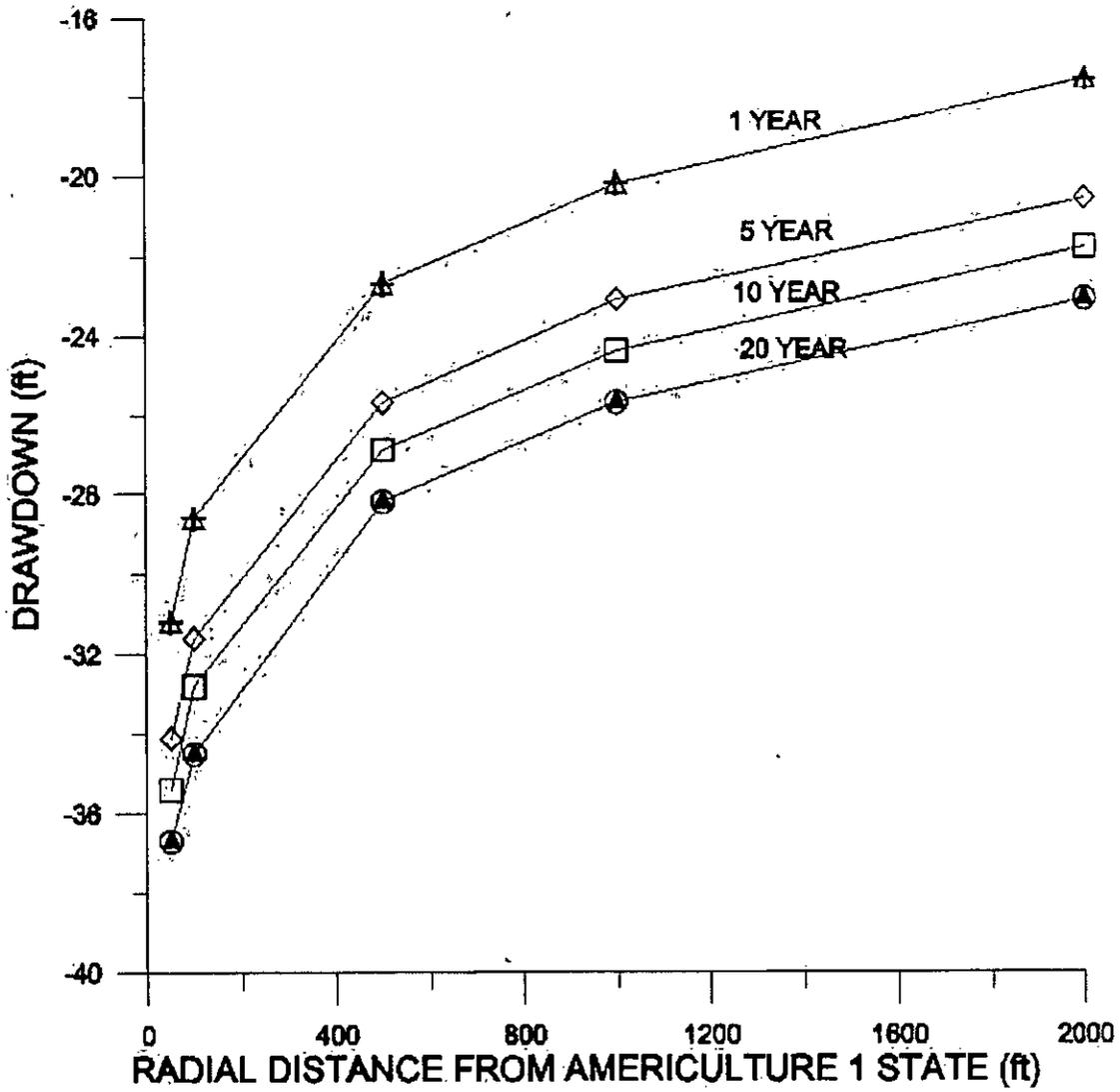
Figure 12. This model drawdowns for the Americulture 1 State well at various times and radial distances.
