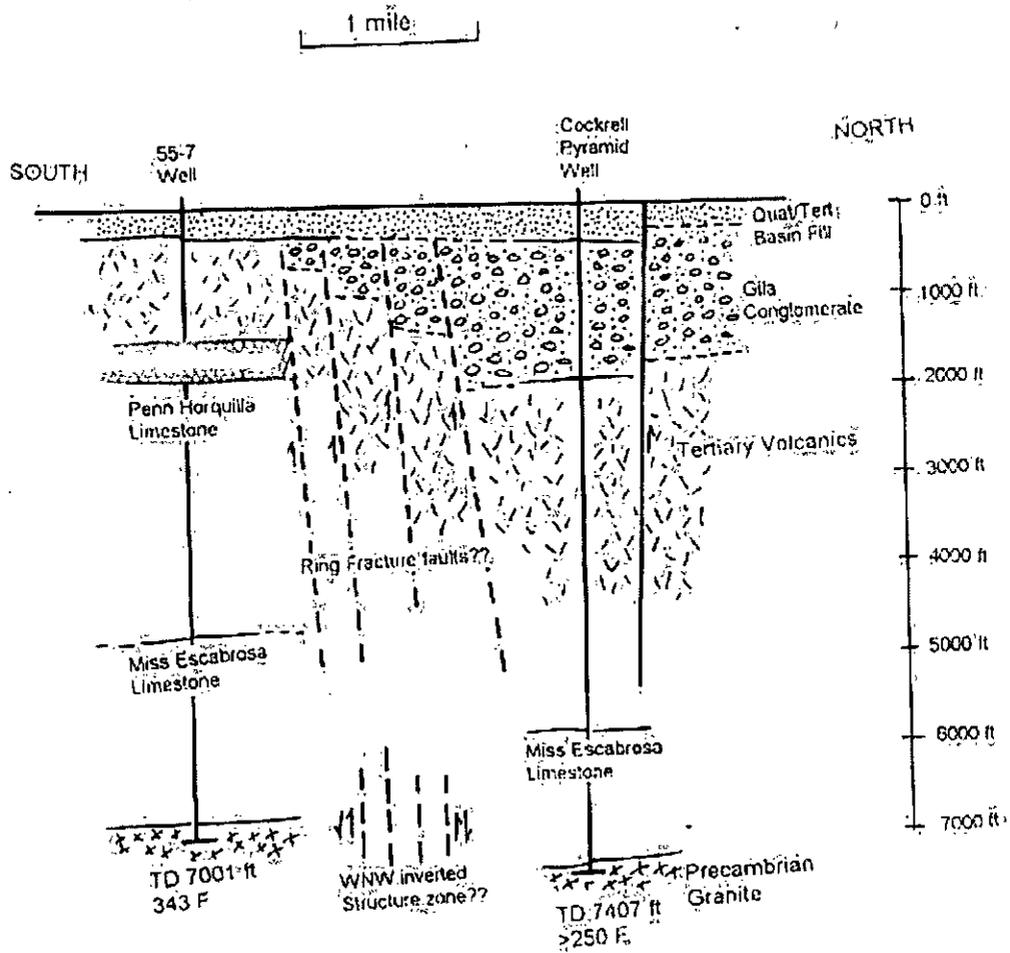
Figure 3. Geologic cross section of the Lightning Dock geothermal area. Deep subsurface control is from the Steam Reserve Animas 55-7 well and the Cockrell Pyramid well.
