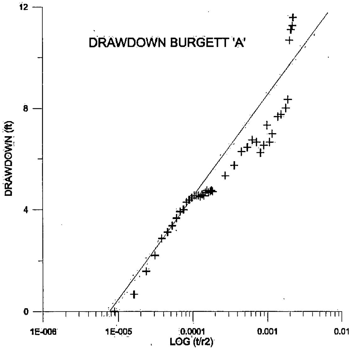
Figure 11. "Best Pick" straight line drawdown for the Burgett 'A' monitor well. Drawdown in feet is plotted against the log ratio of time (minutes) and the distance (825 ft) squared from the pumping AmeriCulture 1 State well.
