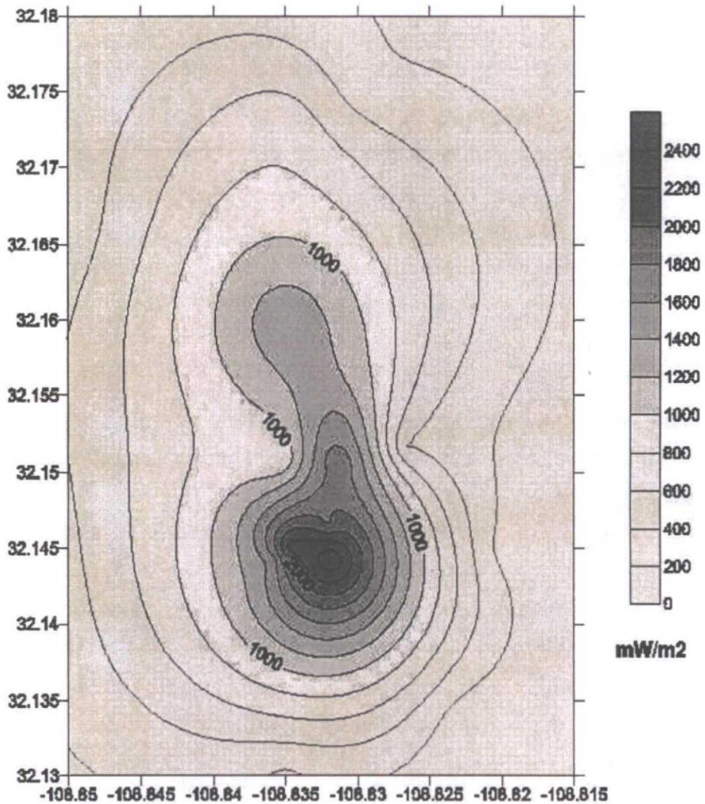
Figure 4. Heat flow map of the Lightning Dock geothermal system. Contour interval is 200 mW/m<sup>2</sup>.
