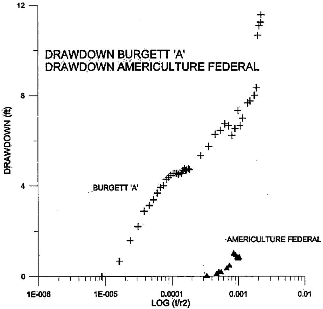
Figure 10. Comparative drawdown for monitor wells Burgett 'A' and AmeriCulture Federal. Drawdown in ft is plotted against the log ratio of time (minutes) and the distance (ft) squared from the pumping AmeriCulture 1 State well.
