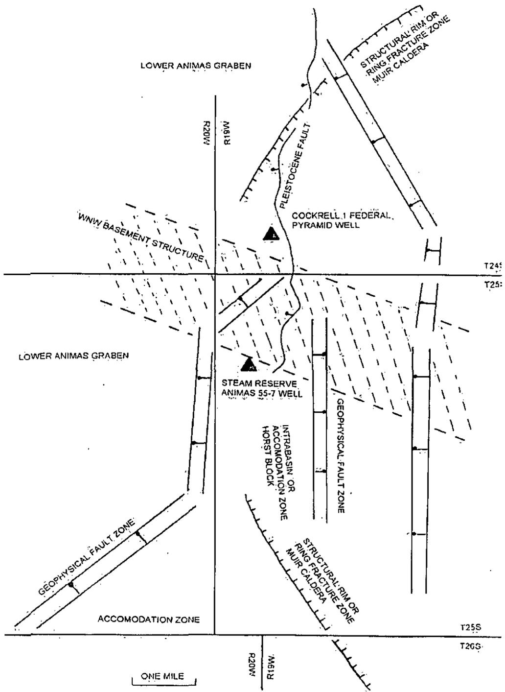
Figure 2. Summary geologic structure map of Lightning Dock geothermal area.
