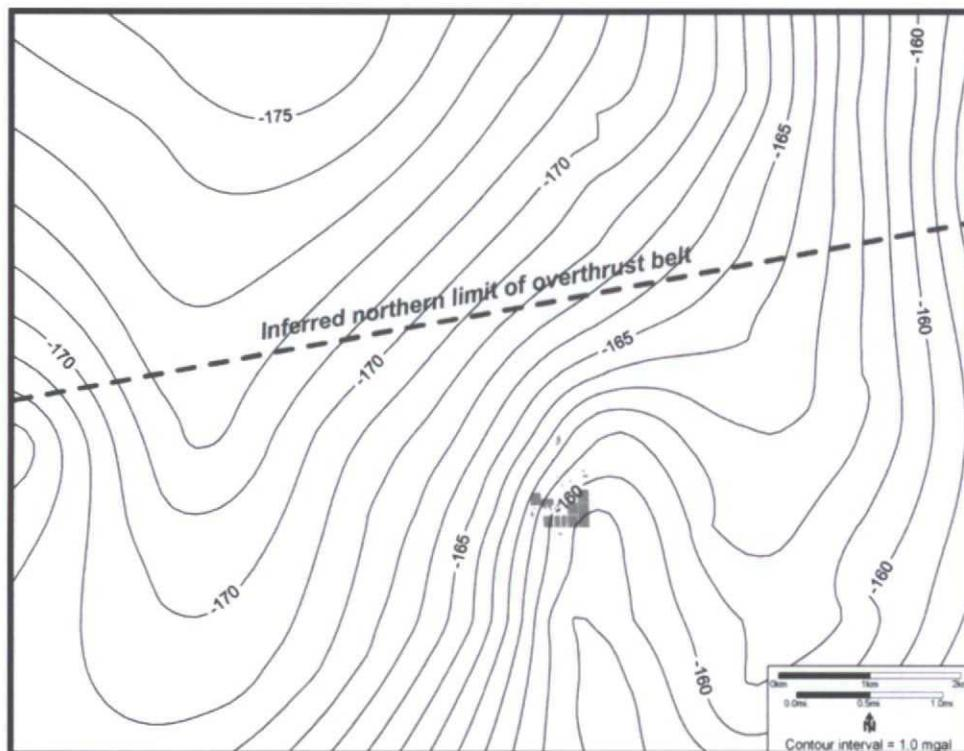
Figure 4. Simple Bouguer gravity contours.
