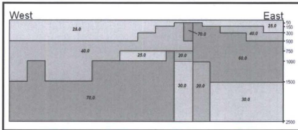
Figure 6. Resistivity block model for the Caliche Road line (from Mackelprang, 2001).
