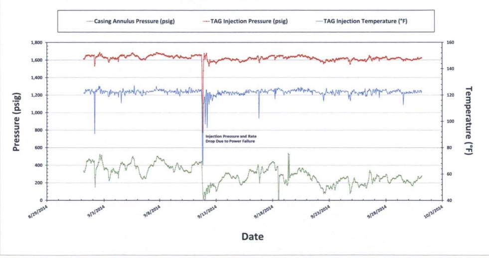
Linam AGI #1 TAG Injection Pressure and Casing Annular Pressure Differential (psig) 9/1/2014 to 9/30/2014
