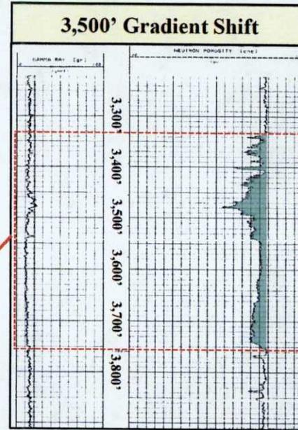
Temperature gradient shifts correspond to intervals where the lithology shifts, penetration rate decreases, and cased hole neutron shows variations.
