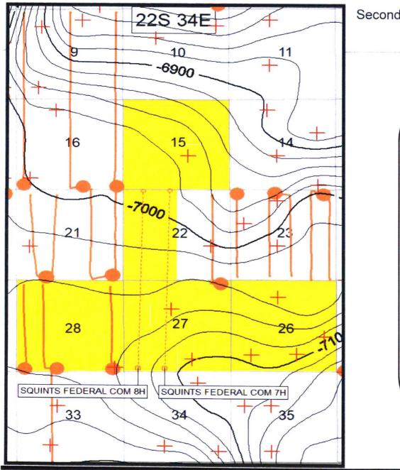
Second Bone Spring Sand Base Subsea Structure Map Squints Federal Com 7H & 8H Section 27 T22S-R34E Map Legend SHL **COG – SBSG Horizontal Location** BHL **Producing SBSG Wells COG** Acreage Data Point **WFMP** Structure CI: 25'
