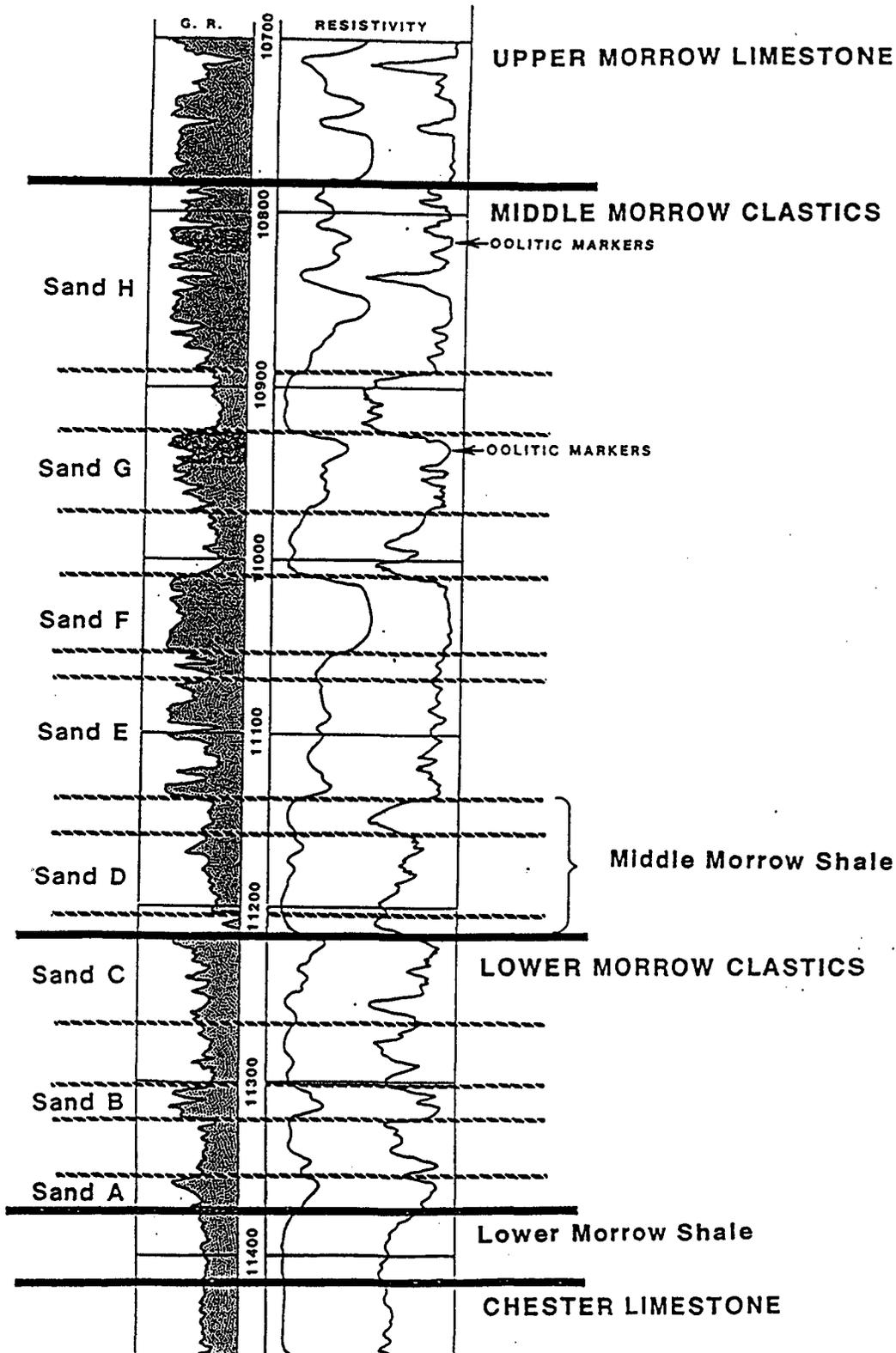
Fig. 11 Type log of the Morrow Clastics in the White City Penn Gas Pool. The well log is the discovery well, the White City Penn Com. 1 No. 1, located in NW/4 of Sec. 29-T24S-R26E. Differentiated are the major Morrow intervals and various sand-rich parasequences. Oolitic marker beds are indicated by a darker stipple pattern.
