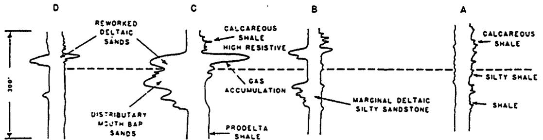
An electric log cross section showing the lateral variation of sandstones in the reworked deltaic setting. This cross section is keyed to the lithologies in above. (After Saxena, 1979)
