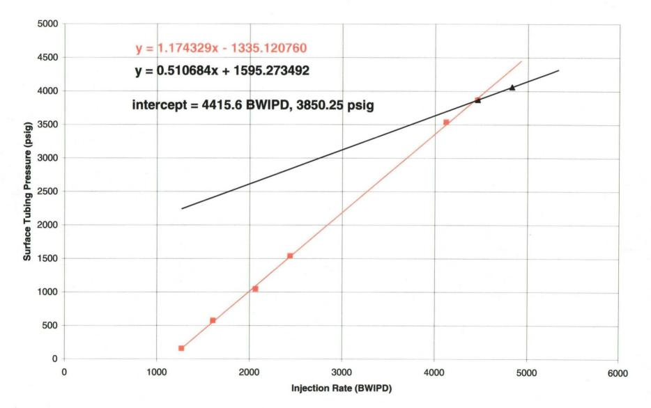
Step Rate Test, Raw Data (NVAWU #3H)
