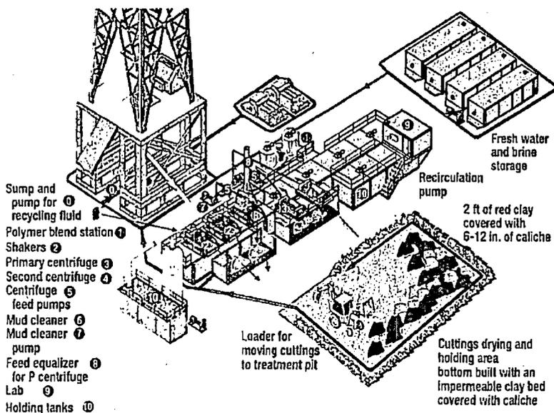
Fig. 2. Schematic of the closed loop dewatering layout used in New Mexico. The key components are the pad, frac tanks for reserve and recycled fluids, cement handling, and the solids control and dewatering equipment.
