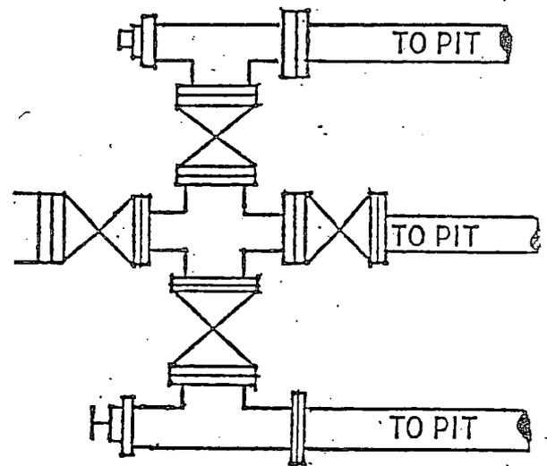
Kill line will be minimum 2" diameter and have 2 valves, one of which shall be a minimum 2" check valve.
