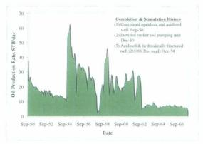
Fig. 7—Well development and completion history, Well TXLSU 1004 (5600 Reservoir).
