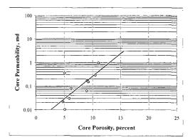
Fig. 6—Core-derived porosity-permeability relationship for rock type 6 (moderate reservoir quality limestone).
