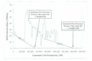
Fig. 8—Estimated ultimate primary moveable oil recovery for Well TXLSU 1004 (5600 Reservoir).
