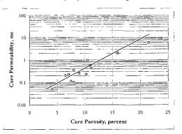
Fig. 5—Core-derived porosity-permeability relationship for rock type 2 (medium crystalline dolo-grainstones).
