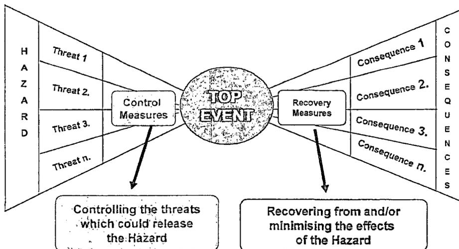
The left side of the Bow Tie, and first step, looks at all causes of that event and the prevention controls. The right side, and second step, of the BTA examines all the potential consequences of the event followed by identification of all recovery measure controls intended to reduce or minimise the loss.
