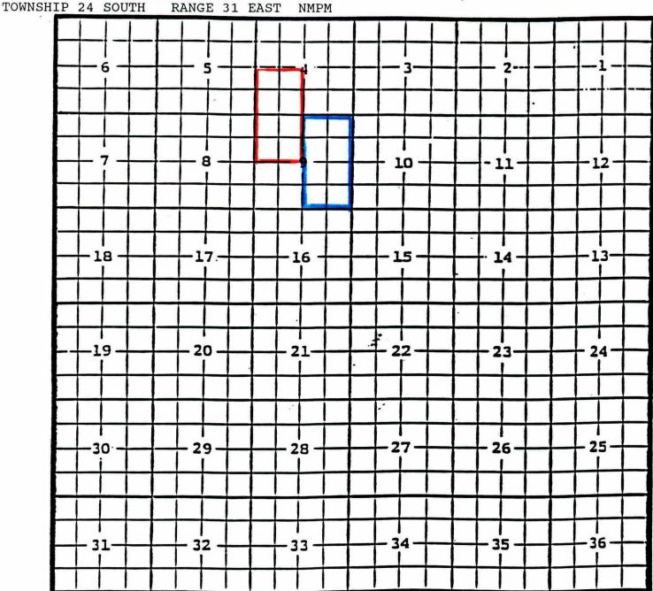
PURPOSE: One completed oil well capable of producing. Bettis, Boyle & Stoval; Lotos Federal No.4 Unit J, Sec.9 T.24., R.31E., NMPM. Completed 12-10-93 in the Delaware formation. Top of perforations are at 8003 feet.
