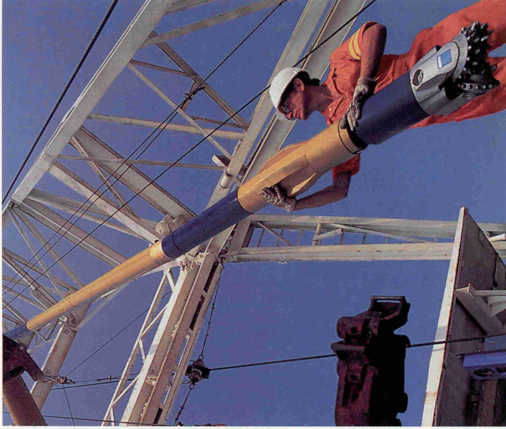
Steerable drilling systems contribute to flexibility in directional drilling.
