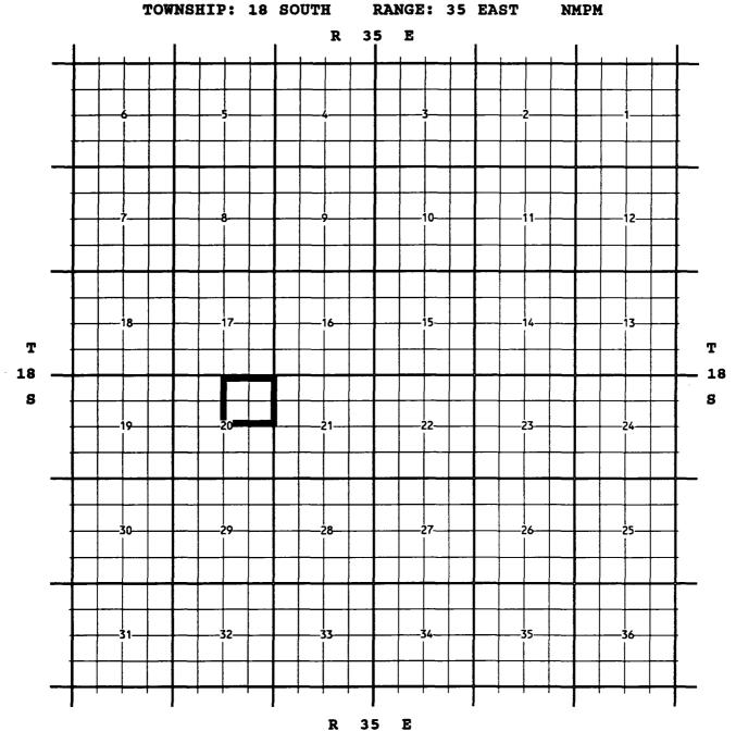
PURPOSE: One completed oil well capable of producing. YATES PETROLEUM CORPORATION, PAWNEE APW STATE # 1, A-20-T18S-R35E, completed 12/31/1996, in the San Andres Formation, top perfs 5140 ft.
