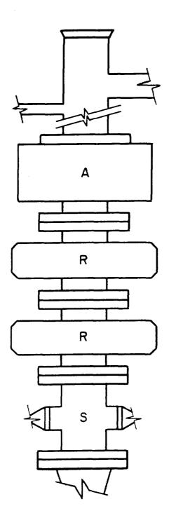
A = ANNULAR-TYPE BLOWOUT PREVENTER 11-inch throughbore, 3000-psi working pressure
