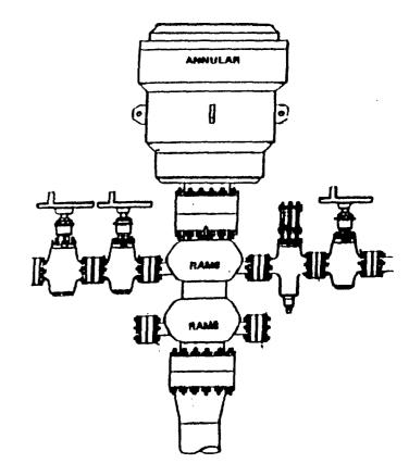
B.O.P. Equipment inlended for use on Rig # 24 Well To Be drilled for <u>Twise</u> (Sharp 'All Volves (H28)' **Choke Manifole:** Pressure Rating 3,000 or 5,000 (as Req.) 1 - 4" Valves 2 - 2" Valves 2 - 2" Valves 2 - 2" Adjustable Chokes Valve Types Used: Cameron - F or FC Shaffer - B Floseal WKM - type 2 Chokes - Cameron H2 or TC unibolt
