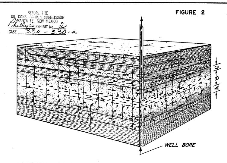
SCHEMATIC DRAWING OF MESA VERDE SANDSTONES AND WELL BORE SHOWING FLOW OF GAS IN RESERVOIR WITH WELL PRODUCING.
