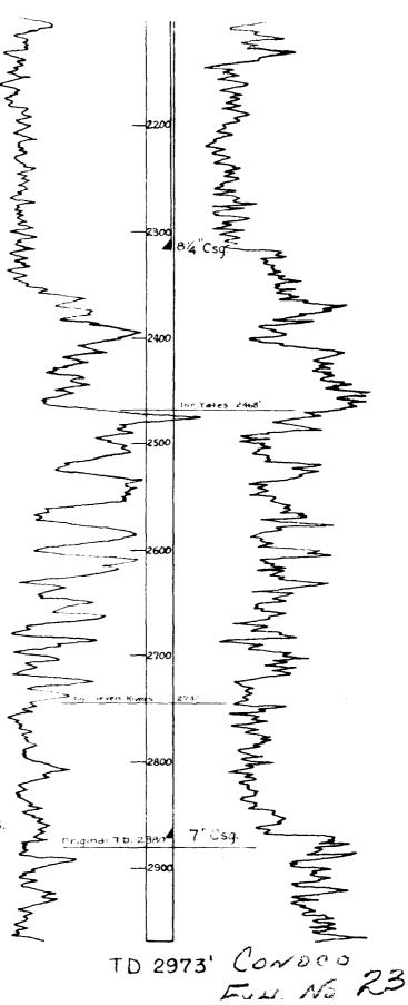
Comp 5-6-28@ 2880'TD, IP 240 Bbls. oil /hr., no water, from open hole 2316-2880:
