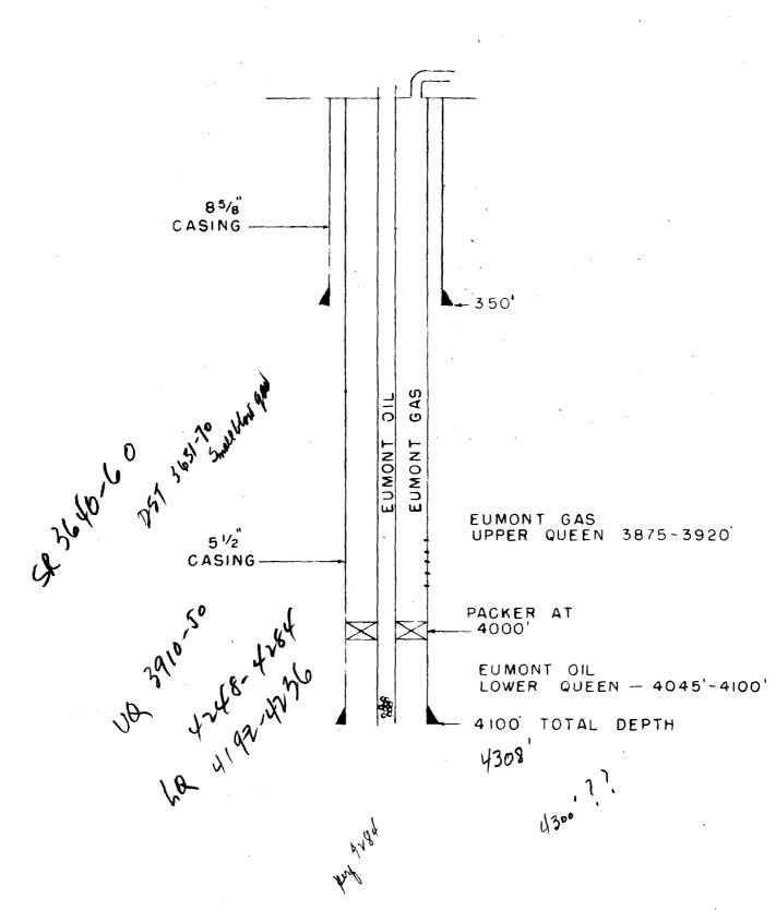
SCHEMATIC DIAGRAM OF PROPOSED DUAL COMPLETION HUMBLE - NEW MEXICO STATE "AO"
