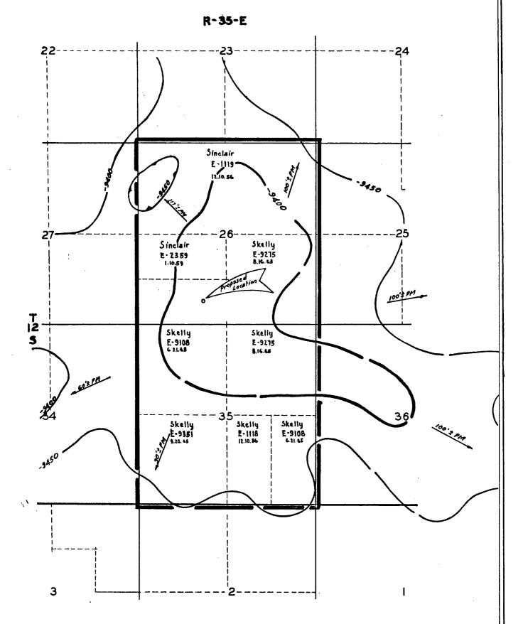
STRUCTURE MAP SEISMIC INTERPRETATION NEAR DEVONIAN HORIZON EXHIBIT "C" SKELLY OIL COMPANY-OPERATOR
