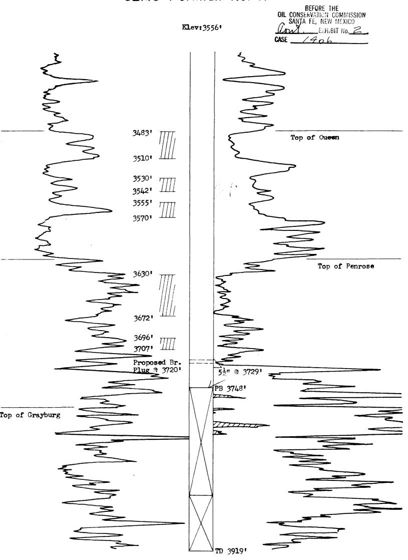
Completed, 1-22-52, @ TD 3919' for 11 BOPD, no water, flowing thru 1" choke.
