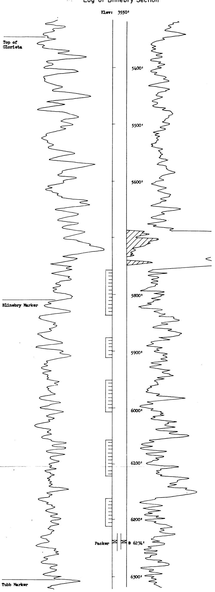
Dual Completion in Blinebry, 2-15-57, for IP of 7650 MCF gas, calculated open-flow, and 147 BDistPD thru open choke with GOR 31,816.
