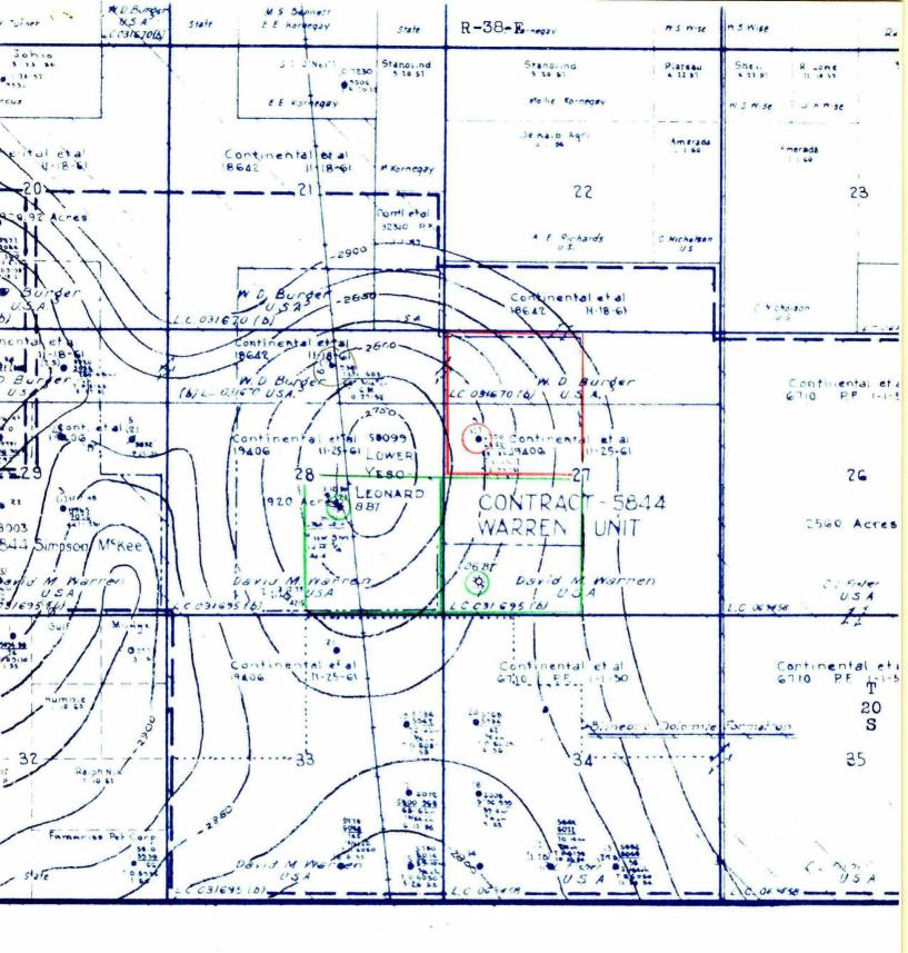
STRUCTURE MAF - TUBB AREA Contoured on Top of Tubb Marker Contour Int: 25' Scale: 1"=2000'
