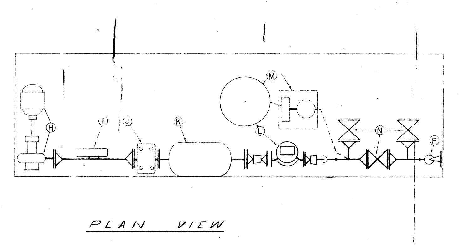
DETAIL SCHEMATIC DIAGRAM OF METERING SKID SOUTH VACUUM AUTOMATIC CUSTODY TRANSFER SYSTEM SOUTH VACUUM UNIT-LEA COUNTY, NEW MEXICO
