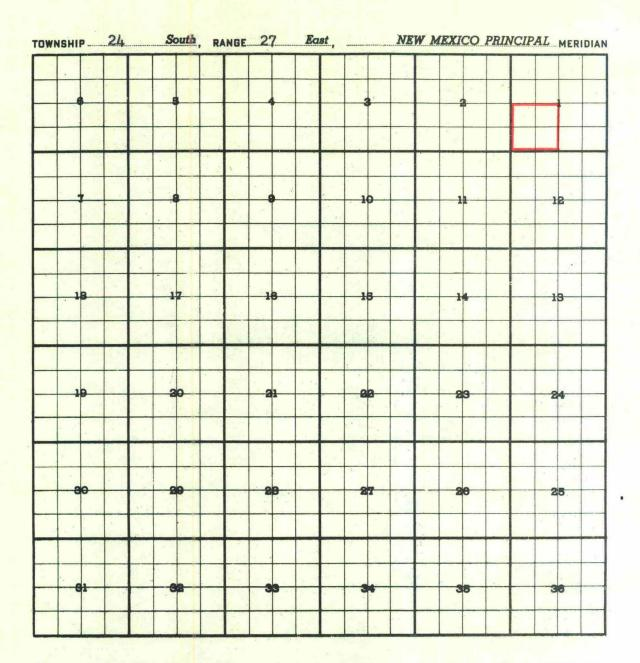
Discovery Well: Ford Chapman & W. D. Thorn et al - State #1 in Unit K of Section 1-24-27. Completed in Delaware formation on March 21, 1958. Top of perforations 2447<sup>\*</sup>.
