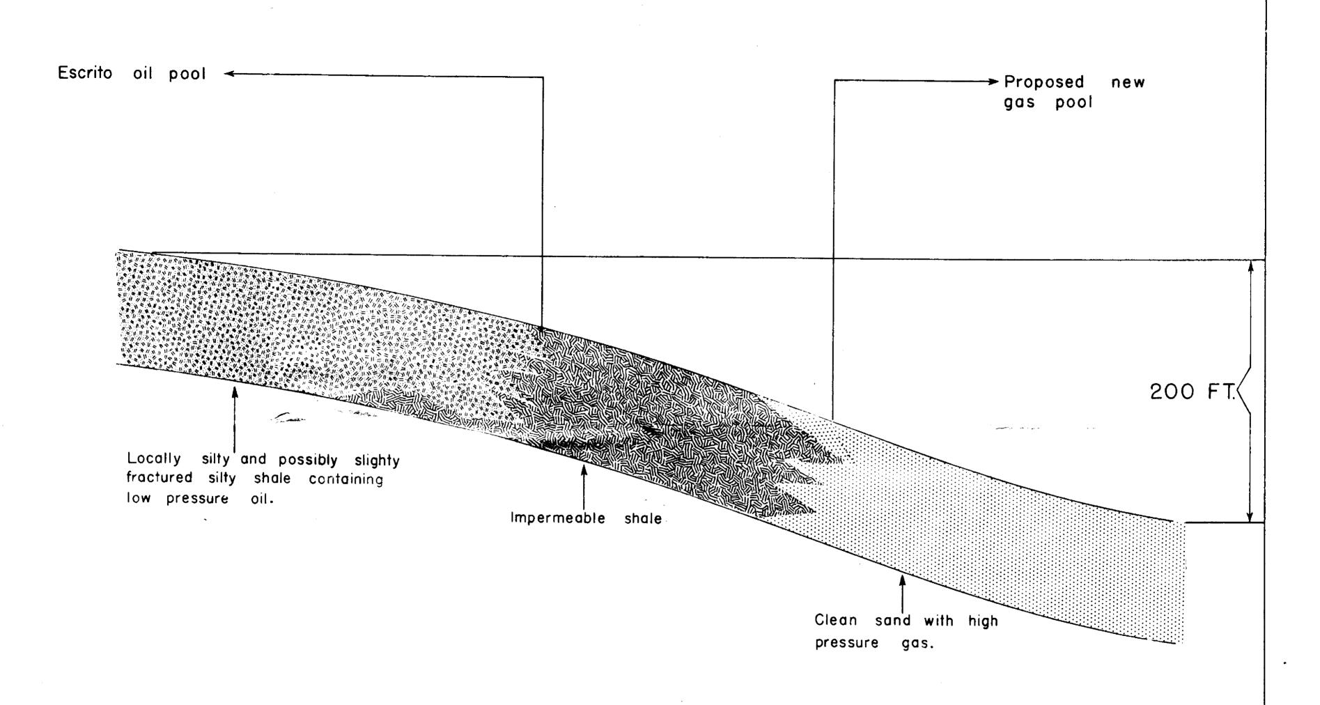
Simplified Diagrammatic Cross Section illustrating clean sand changing to shale facies updip, creating a barrier between Proposed New Gas Pool and Escrito Oil Pool.
