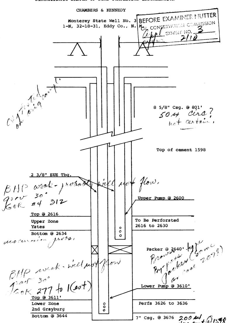
NOTE: Well to be pumped with two strings of rods and two units. Tubing, packer, and pump depths are approximate.
