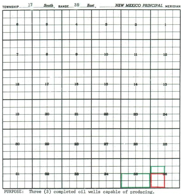
CITIES SERVICE PETROLEUM CO. - State BJ No. 1, Unit I, Section 35-T17S-R35E. Completed in Abo April 3, 1961. TOP OF PERFORATIONS 8914'. ADDITION---CITIES SERVICE PETROLEUM CO. - State BJ No. 2, Unit K, Section 35-T17S-R35E.
