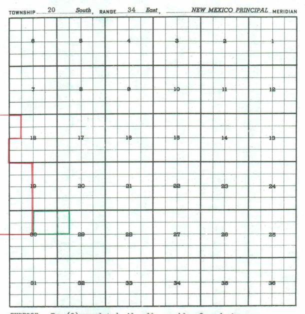
PURPOSE: Two (2) completed oil wells capable of producing. EARL G. COLTON - Wills Federal #1 in Unit D of Section 29-20-34. Completed in Yates September 4, 1961. TOP OF PERFORATIONS 3356'. GACKLE DRILLING CO. - Texaco Federal #1 in Unit A of Section 30-20-34. Completed in Yates August 13, 1961. TOP OF PERFORATIONS 3326'.
