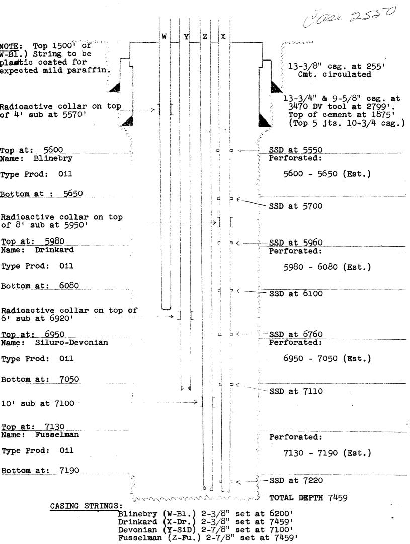
NOTE: Cementing to be accomplished by cementing through (X-Dr.), (Y-SiD) and (Z-Fu) strings with approximately 1150 sacks of cement. Calculated top of cement at 2800'. Primary cementing to be supplemented by squeeze cementing through Otis Type "A" Sliding Side Doors (SSD).
