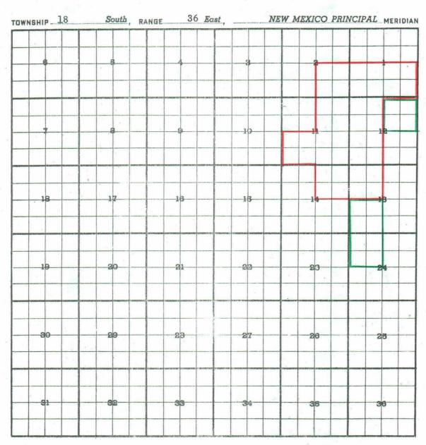
PURPOSE: Two (2) completed gas wells capable of producing. W.K. BYROM-State 24 No. 2 in Unit D of Section 24-18-36. Completed in Queen March 3, 1962. Top of Perforations 4430' CACTUS DRILLING COMPANY-U. S. Smelting No. 1 in Unit G of Section 12-18-36. Completed in Queen March 25, 1962. Top of Perforations 4442 Pool boundary colored in red. Proposed extensions colored in green. SECTION 12: NE/4
