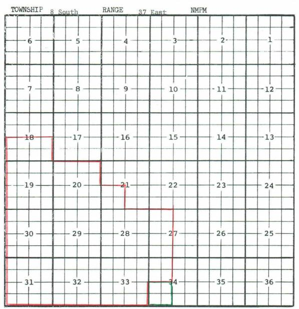
PURPOSE: one completed oil well capable of producing. DOB OIL PROPERTIES, INC. - Humble Federal #1 in Unit L of Section 34-8-37. Completed in Pennsylvanian on January 16, 1963. Top of Perforations 9581'. Pool boundary colored in red. Proposed extension colored in green. SECTION 34: SW/4
