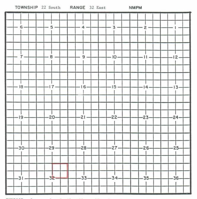
Yates Petroleum Corporation Lotus ALT State Well No. 2 located in Unit G of Section 32, Township 22 South, Range 32 East, NMPM. It was completed October 19, 1992, in the Delaware formation. The top of the perforations is at 8,326 feet.
