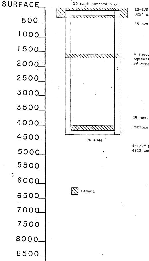
13-3/8" surface casing set at 322' with cement circulated
