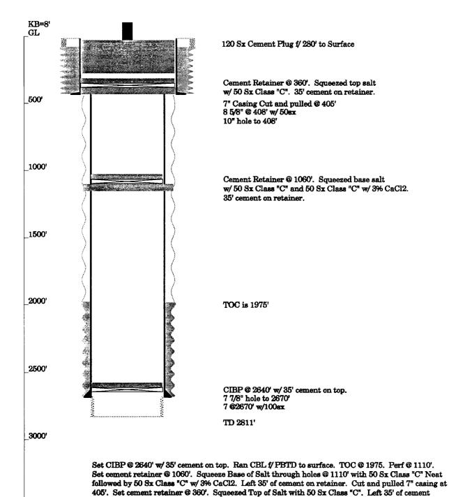
on top of the retainer. Spot 120 Sx plug from 280' to surface. Allow to work behind 7" casing through
