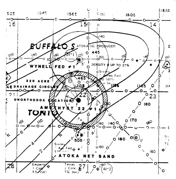
Assume drainage area is directly proportional to flow rate. Drainage circles are shown for Sante Fe's unorthodox location using several penalties as follows:
