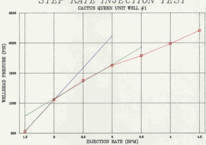
STEP RATE INJECTION TEST
