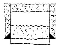
85/8" 23" casing set @ 300' in 12 3/4" hole with 250 sx. Cmt Circ.
