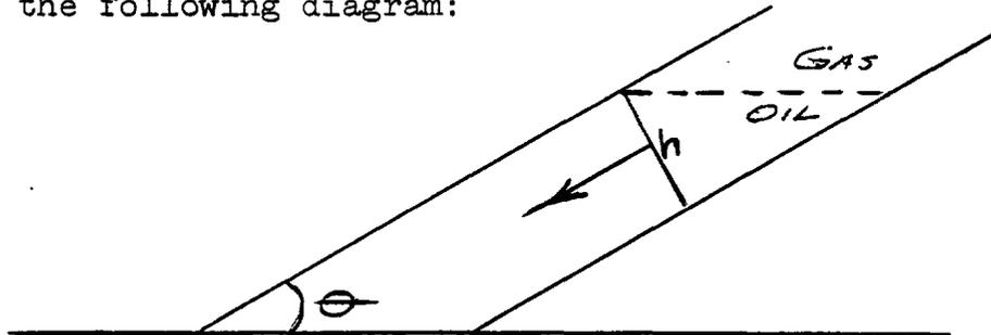
With reference to the above sketch, we may determine the surface area of gas-oil contact to be: *(per linear mile along the strike)*
