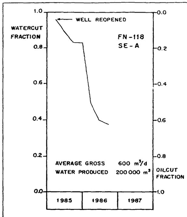
Fig. 14—Typical recent water-cut performance of a Reservoir SE-A completion.
