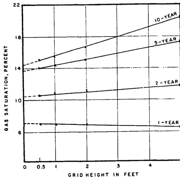
Fig. 3—Effect of grid height on gas saturation.
