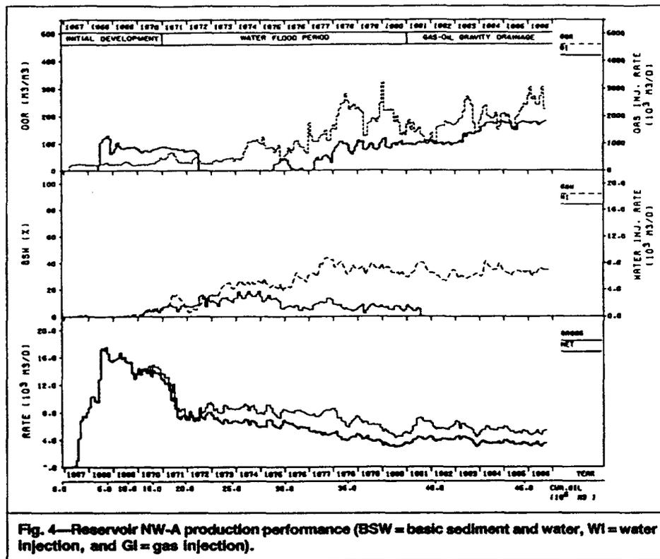
Fig. 4—Reservoir NW-A production performance (BSW = basic sediment and water, WI = water injection, and GI = gas injection).
