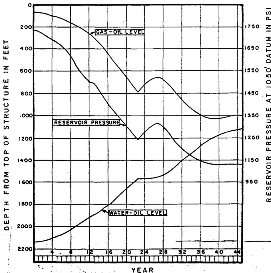
Fig. 4—Pressure, gas-oil and water-oil levels of the Haft Kel.
