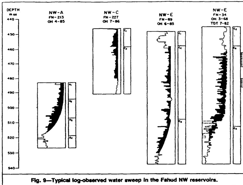
Fig. 9—Typical log-observed water sweep in the Fahud NW reservoirs.
