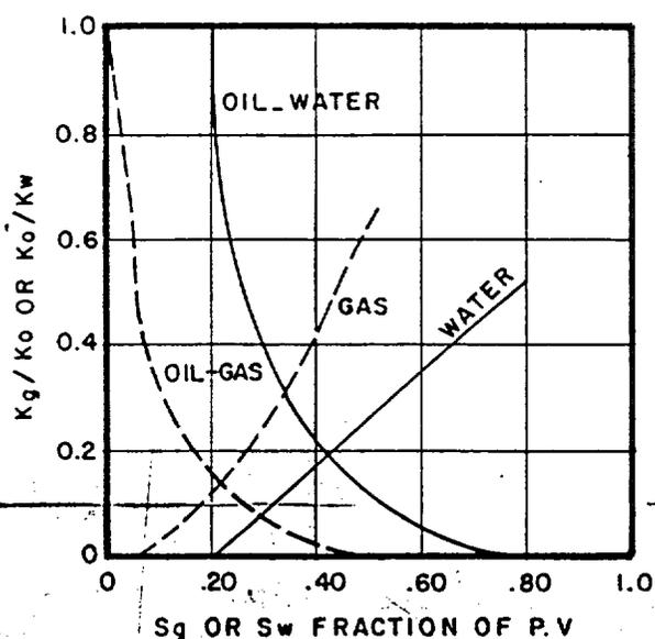
Fig. 5—Oil, water and gas relative permeability.
