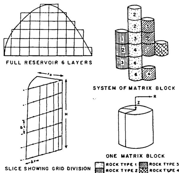
Fig. 1—Schematic representation of a reservoir by the model.
