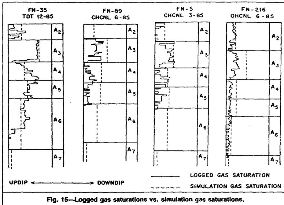
Fig. 15—Logged gas saturations vs. simulation gas saturations.
