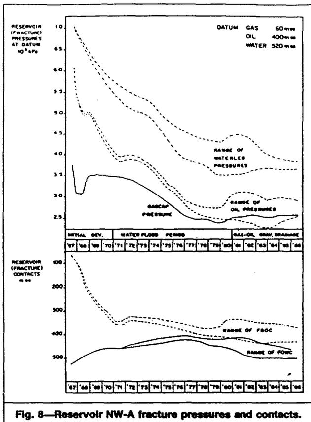
Fig. 8—Reservoir NW-A fracture pressures and contacts.
