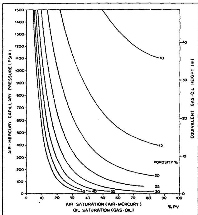
Fig. 13—Air/mercury capillary pressures and equivalent gas/oil height.
