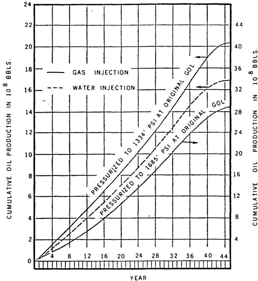
Fig. 8—Oil recovery under different fluid injection schemes.
