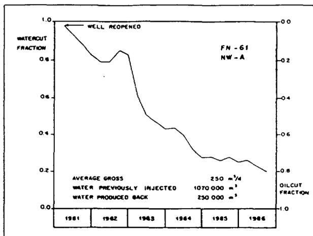
**Fig. 12—Typical recent water-cut performance of a Reservoir NW-A completion.**
