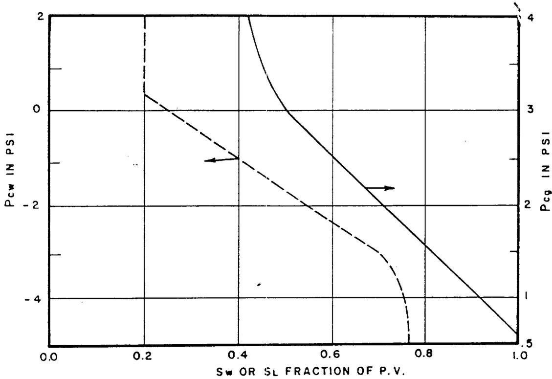
Fig. 6—Average water-oil and gas-oil capillary pressure used for Haft Kel Field.
