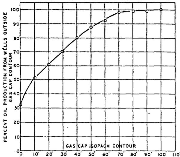
Fig. 6 - Distribution of oil production with respect to gas-cap thickness.
