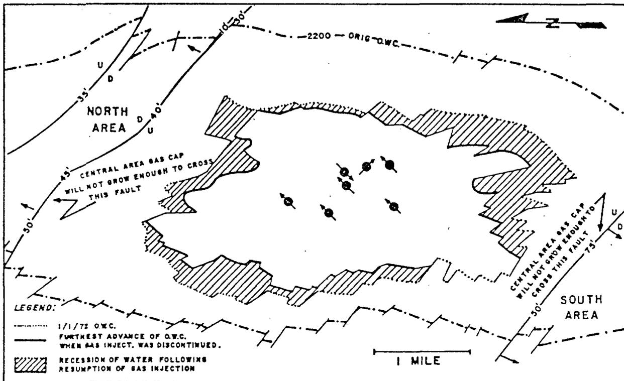
Fig. 4— Effect of resumption of gas injection.
