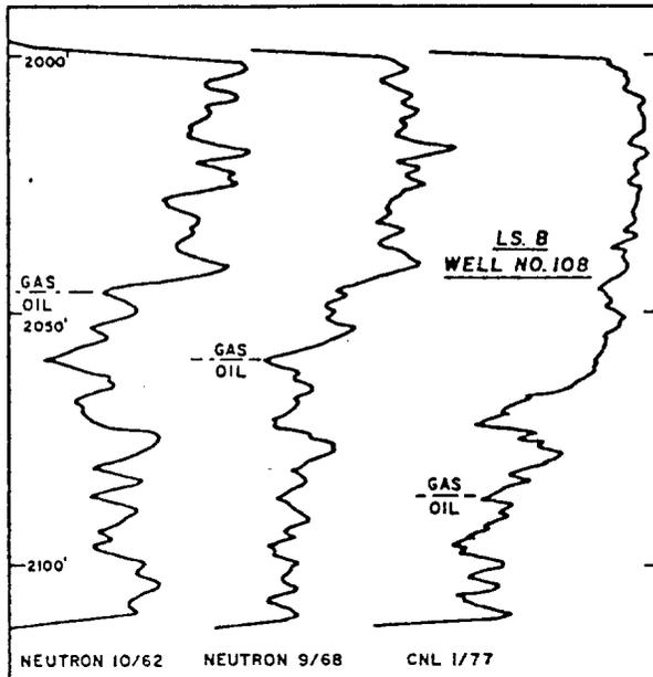
Fig. 11 – Monitoring gas-cap advance by neutron logs.
