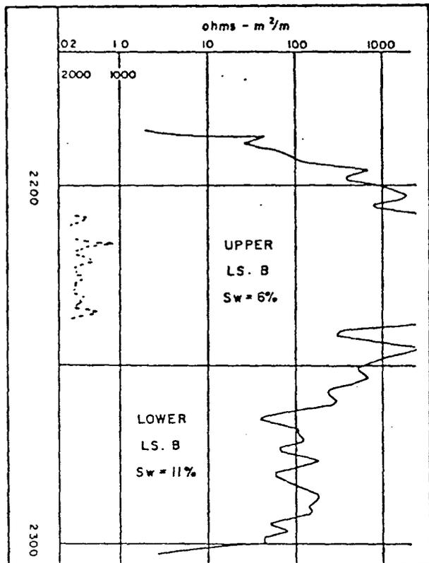
Fig. 13 - Typical Laterolog of Limestone B original oil column.
