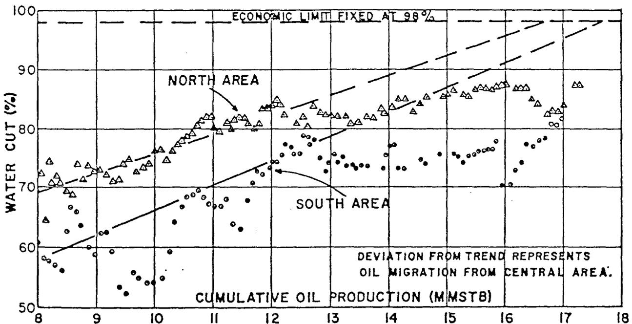
Fig. 10 - Cumulative oil production vs water cut.
