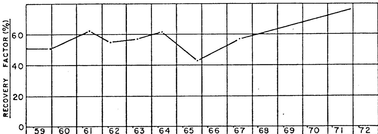
Fig. 12 – Oil recovery factors by gas displacement (based on data obtained from neutron and pressure surveys).
